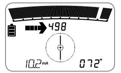
Figure one shows the locator in Guidance Mode with the locator positioned to the left of the target line. In this position the Proportional Left arrow is displayed, indicating the direction in which the locator should be moved towards the target line. The target position indicator indicates the target positioned to the right of the locator and
