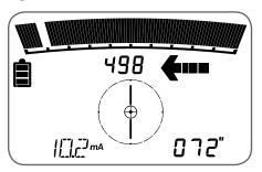
Figure three shows the locator in Guidance Mode and positioned to the right of the target line. In this position the Proportional Right arrow is displayed, indicating the direction in which the locator should be moved towards the target line. The target position indicator indicates the target positioned to the left of the locator and can be used to
