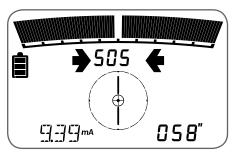
Figure two shows the locator in Guidance Mode and directly over the target line. In this position the left and right arrow heads will be displayed simultaneously, target position indicator in the centre, the signal strength value at its maximum, speaker tone silent and both depth and current readings at their minimum.
