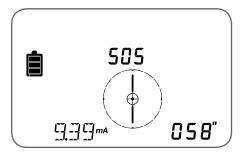
With the locator powered up, a momentary press of the On/Off key will change the mode of operation to Signal Strength Mode. In this mode, the compass, signal strength, depth and current will be available. The proportional left/right arrows and target position indicator will not be available. See figure four.
